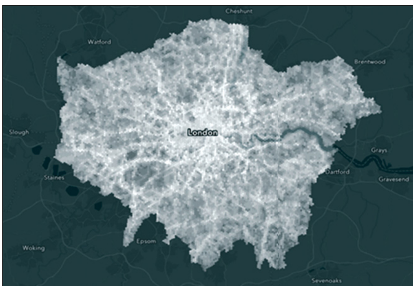
Figure 1: Illustrates the user interface of the Green Infrastructure Focus mapping tool. The following map shows the composite score for London, based upon factors such as, but not limited to, air quality, pedestrian activity, and access to public open space. The lighter areas reflect which areas are currently underserved.
